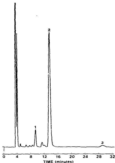
Fig. 2. HPLC chromatogram of DNB derivatives of neomycin using a 5- \mu m particle size silica column. Mobile phase: chloroform-THF-water (600:392:8). Peaks: 1 = neomycin C; 2 = neomycin B; 3 = mono-N-acetylneomycin B (LP B ).
